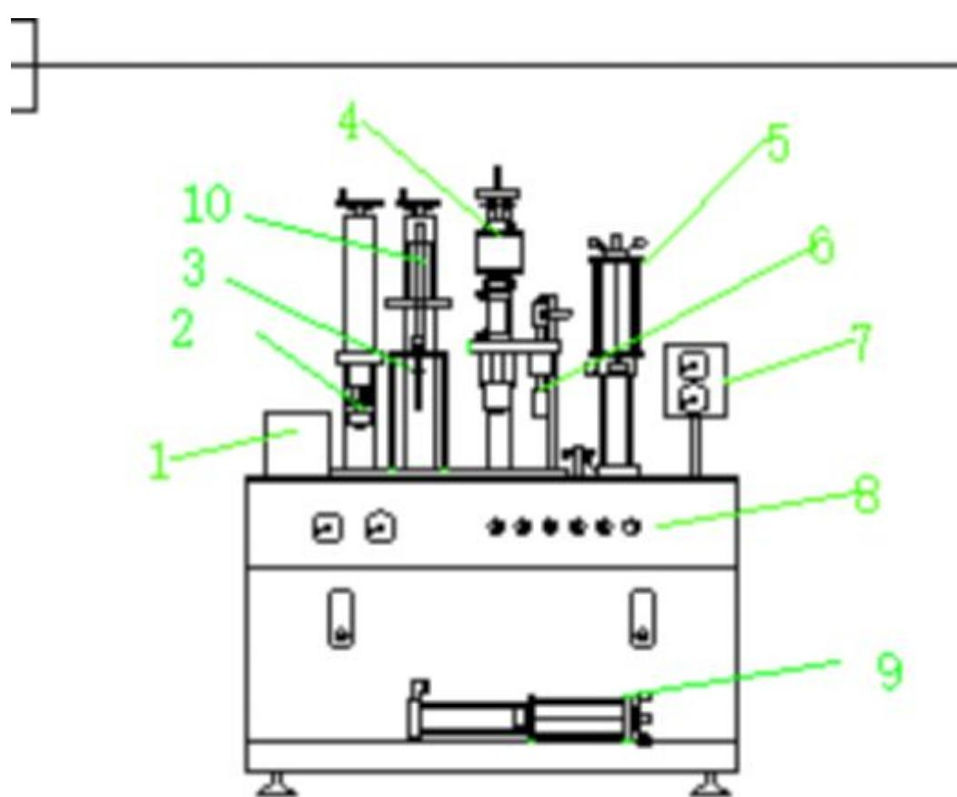
1.transfer system 2.liquid filling head 3.automatic valve 4.sealing cylinder 5.gas filling head
